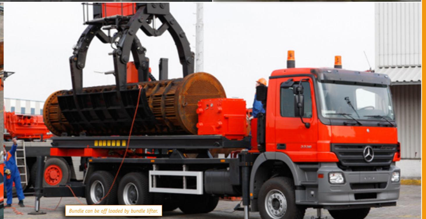
Standard supplied with a 6 x 4 Mercedes or Volvo truck. The system can also be fitted on US truck like Peterbilt.
