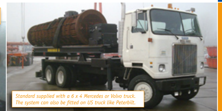
Hydraulic axle locking system for optimal safety during bundle transport prevents the truck from tipping over
